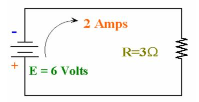
We have introduced a new schematic symbol here too. The schematic symbol of a battery is shown at the left. Note the small bar at the top is the negative terminal. The direction of current flow is shown correctly, from negative to positive
